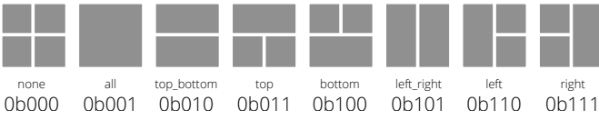
Fig. 6. Merge modes of the irregular grid: There are eight possibilities of merging adjacent cells to form a cell with rectangles.
