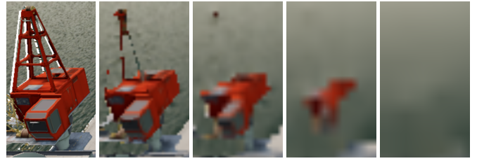
Fig. 9. This example shows five different levels of the filtered image pyramid. Holes and the foreground object dissolve in higher levels because only non-hole pixels and pixels with a depth larger than the kernel average are taken into account for filtering.
