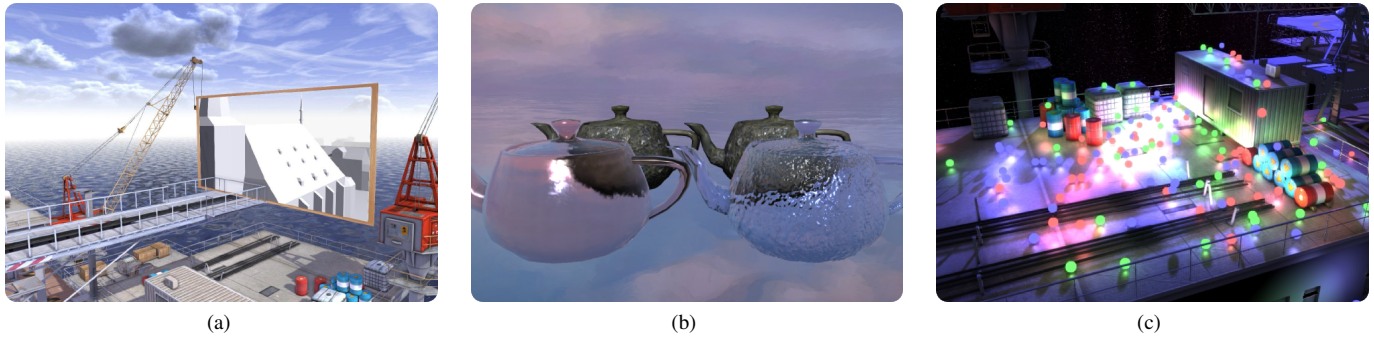
Fig. 7: In image (a), the combination of two pipelines is used to create a portal which shows a view into another virtual scene. The first pipeline is rendered to a texture which is then used by the second pipeline. Image (b) shows the use of multiple pipelines for advanced material effects. In this example, the illusion of refraction is achieved by using a pipeline’s result as input for the glass material. The very large amount of small light sources shown in image (c) demonstrates one advantage of deferred lighting.
